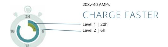
Depending on the battery technology used in the vehicle, Level 2 charging generally takes 4–6 hours to completely charge a fully depleted battery.
